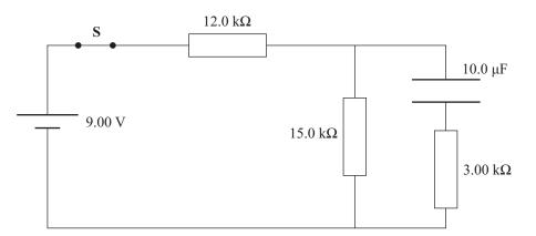
(a) (i) Calculate the steady-state current in each resistor.
