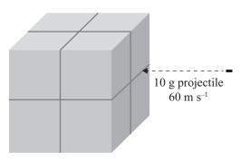
(a) Show that once the projectile stops, the velocity of the centre of mass of the cube and projectile is  $0.74 \text{ m s}^{-1}$ .
